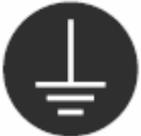
Indicates a "Protective Earth Terminal." Before operating the equipment, be sure to connect it to the Ground.
